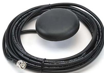
The bolt mount antenna is ideal for permanent installations and enables the antenna system to be securely affixed in location. The cable supplied is the maximum specified length to avoid any loss of signal and maintain call quality. It is not recommended to extend this cable further to avoid loss of dB beyond the specification.
